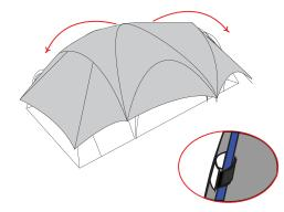
**7.** Pull the fly over the inner tent. The Zempire logo should be at the front and rear of the tent. Connect the velcro loops inside the fly around the cut outs on the corresponding pole sleeve.
