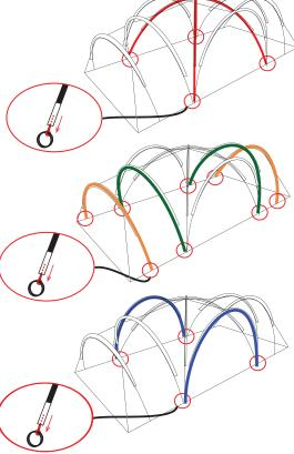
**6.** Peg out all the peg points around the inner tent. The peg points at the base of each pole should be pegged through the webbing loop rather than the steel ring.
