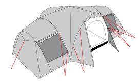
**9.** It is recommended that guy ropes are pegged out at all times and windows are opened whenever possible to allow adequate ventilation. Try to have the guy ropes at 45<sub>0</sub> angle to the ground.
